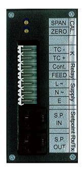
Adjust at both low (ZERO) and high (SPAN) values e.g. 100 and 1000 Deg.C.
